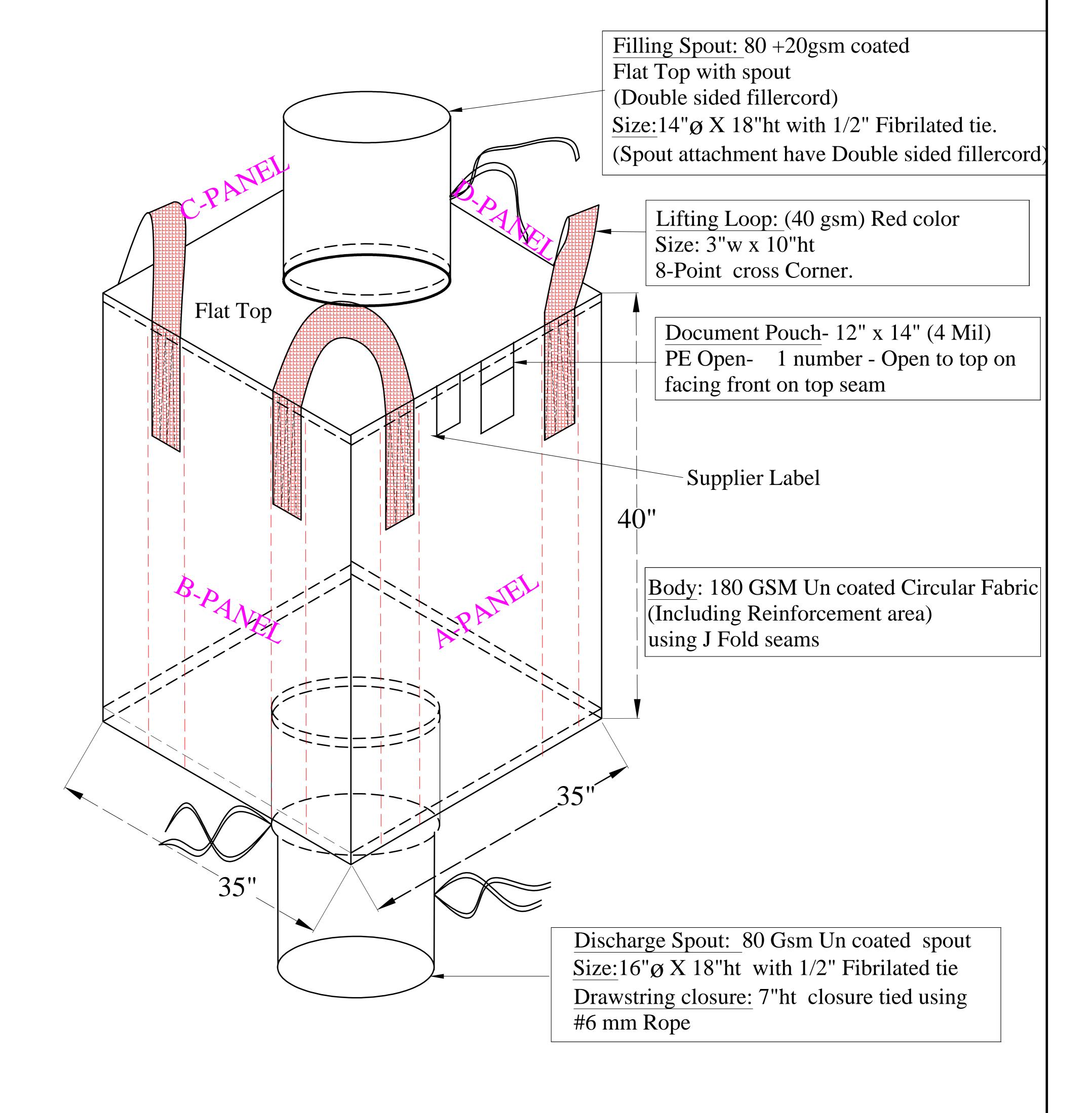
Note:- Inlet Spout attachment have Double sided fillercord. Do not Exceed 22" Layflat on inlet spout
